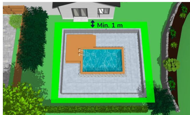
Example of a pool enclosure located more than 1 m from a retaining wall.
