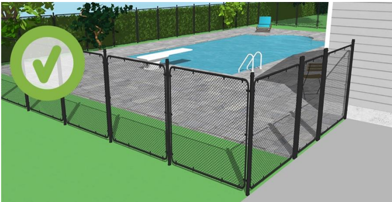
Example of a chain-link fence with a mesh less than 30 mm wide.
