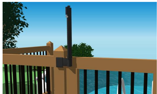
Example of a latch that can be installed on the outside of the side of the enclosure, even when the enclosure is less than 1.5 m high.
