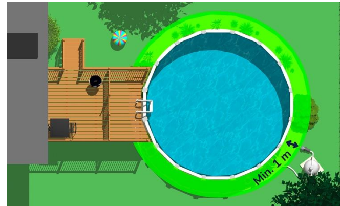
The operating devices of the pools are located at more than 1 m from it. In addition, there is no fixed equipment that can be used to climb over the wall within 1 m of it.
