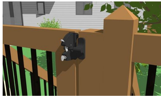
Example of a latch that allows the door to lock automatically . The door should also be equipped with spring hinges to close automatically.
