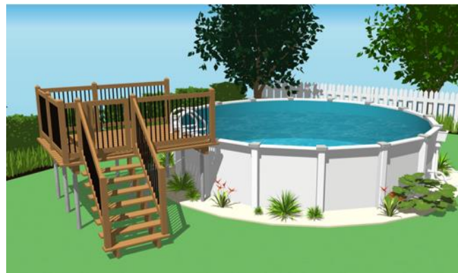
Example of a platform with an access protected by an enclosure.
