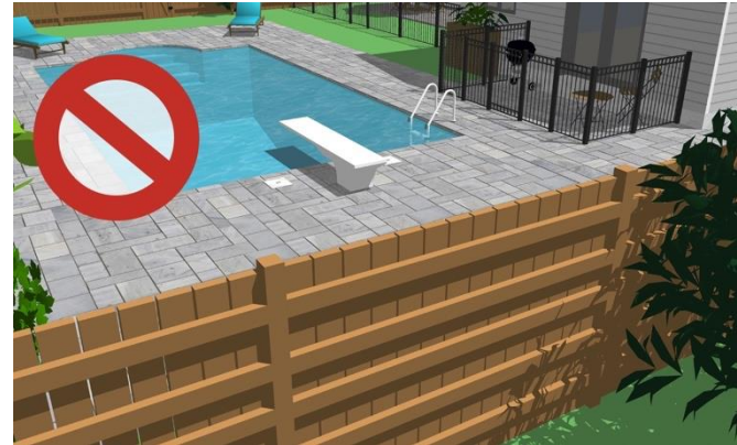
The horizontal rails are too close together and could allow a child to climb the fence.
